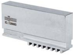
A09 Unstepped jaw BL, special length, soft, 16MnCr5, DIN 6350
