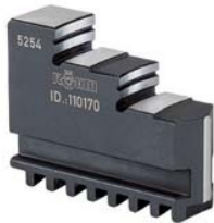
A09 Unstepped jaw BL DIN 6350, unstepped, soft, 16MnCr5
