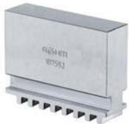
A09 Unstepped jaw BL DIN 6350, unstepped, soft, 16MnCr5
