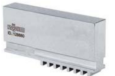
A09 Unstepped jaw BL, special length, soft, 16MnCr5 DIN 6350
