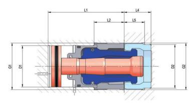
Built-in clamping head RESK, change interface for machine components
