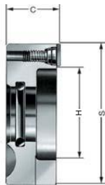
A14 Driving discs, with interchangeable carbide driving plates 6 x 3.2, right- and left-hand rotation
