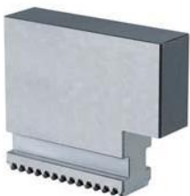
C 21 Soft one-piece jaws, 3-jaw set, can be hardened straight tothing, guidance hardened and ground - material: 16 MnCr 5
