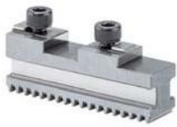
A 36 Reversible top jaws, 3-jaw set, hardened tongue and groove for external and internal clamping - Material: 16 MnCr 5
