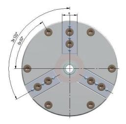
C 15 High-precision air-operated lathe chuck PKF, concentricity 0.003 mm, repetitive clamping accuracy 0.0015 mm with through-hole, pneumatically operated, with integrated pneumatic piston, clamping precision in the  $\mu$  range
